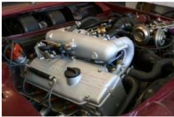
The author's freshly-rebuilt M10-powered 1977 320i.
